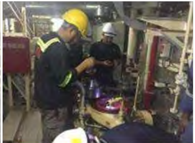
TESTING, COMMISSIONING & HARBOUR ACCEPTANCE TRIAL (HAT) F.O & L.O PURIFIER ONBOARD RMN TRAINING VESSELS GAGAH SAMUDERA AND TEGUH SAMUDERA
