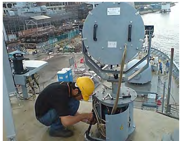
VESSEL SEARCH LIGHT AND CONTROLLER SERVICING & TEST
